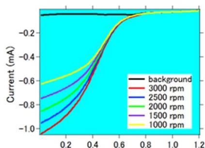
Catalytic measurement of carbon alloy, Current against voltage (rotation speed dependent)
