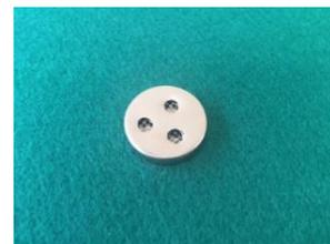
Coin cell type of aluminium air battery
